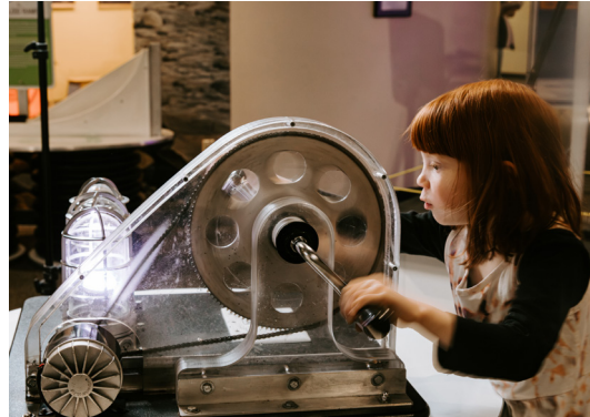
At GEAR UP , 'pedal' a crank to generate power and see how much electricity you can create to make fluorescent, incandescent, and LED bulbs glow.
