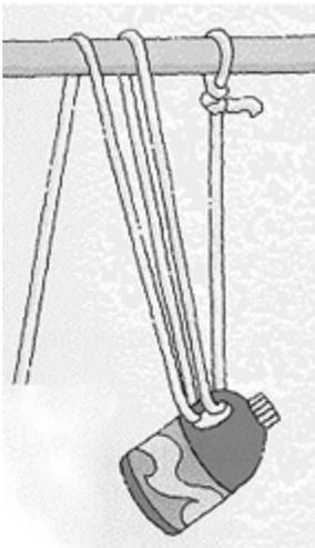
Explanation: Each loop of rope acts as a pulley. The total weight of the jug is distributed among the loops so that each loop holds a portion of the load. To raise the load, the rope has to go a greater distance, but the amount of effort is reduced.
